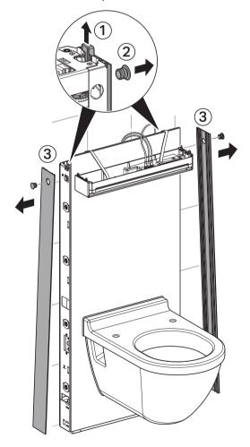
The power supply unit will either be on the right- or left-hand side of the frame, depending on the installation situation.
