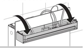
2 Disconnect the plug connections.
