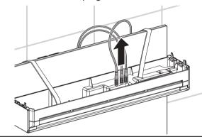
3 Loosen the lid retainers at the frame and replace the cistern lid.
