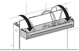
2 Disconnect the plug connections.
