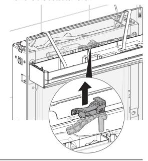
5 Loosen and remove the lower part of the odour extraction unit together with the fill valve.
