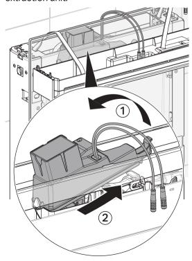
4 Remove the actuator lever.
